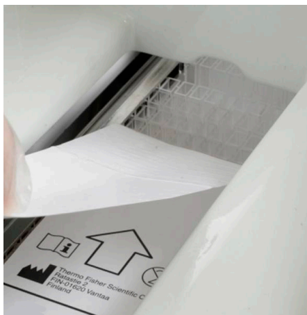
Cuvette loader for 360 cells. Low-volume reaction cuvette uses reagent and water for lower environmental impact.
