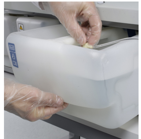
The analyzer is self-contained with no need for external water or drainage connections, which makes the analyzer quick and easy to install.
